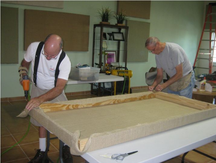
Next, the frame is fitted with a special type of fiberglass designed to absorb sound. You might notice that the fiberglass does not completely fill the frame – there is a bit of an air-space between the fiberglass and the wall which helps absorb the echoes.
